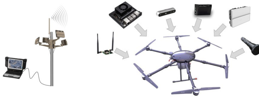
Figure 1: Hardware components of the ground detection and control station (left) and the interceptor UAS (right) [product photos from respective manufactures].
